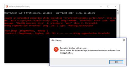
Note how the error line is annotated with the long arrow <------- followed by the message of the error that occured in this line (here: *Wrong segmentation threshold*).
