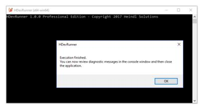
This gives you a chance to review any diagnostic or error messages or the time required for execution in the console before the application closes. If this is not desired, you could either run HDevRunner with the command line argument --no-dialogs or put the exit () operator as last operator in your HDevelop script:
